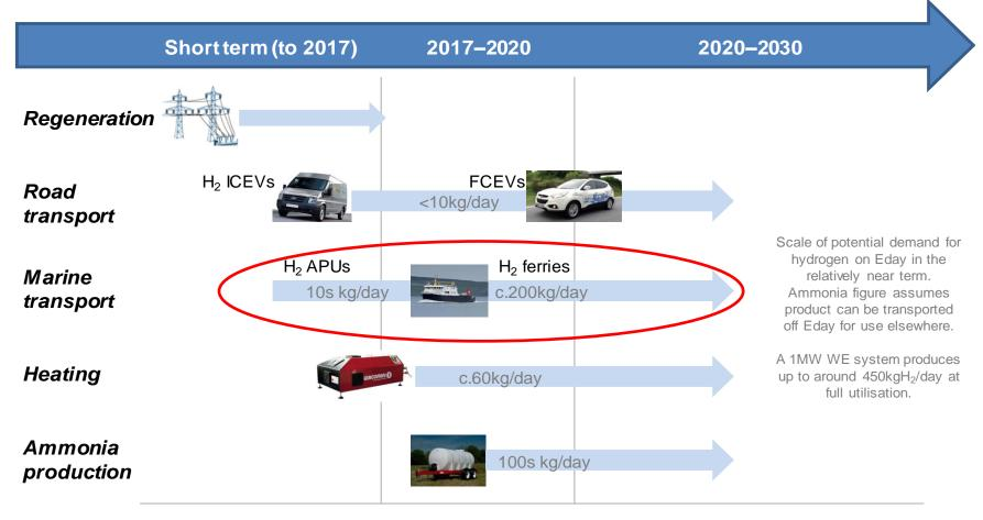
ICEV = internal combustion engine vehicle, FCEV = fuel cell electric vehicle, APU = auxiliary power unit
